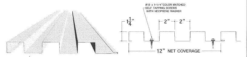
This square rib panel is an exposed-fastener design. With a relatively short span, it offers greater flexibility than most other panels.
